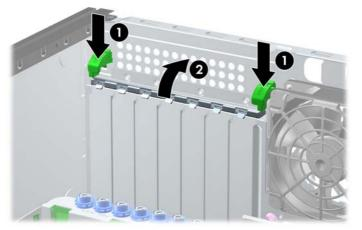
Figure 5-9 Opening the Expansion Slot Retainer
